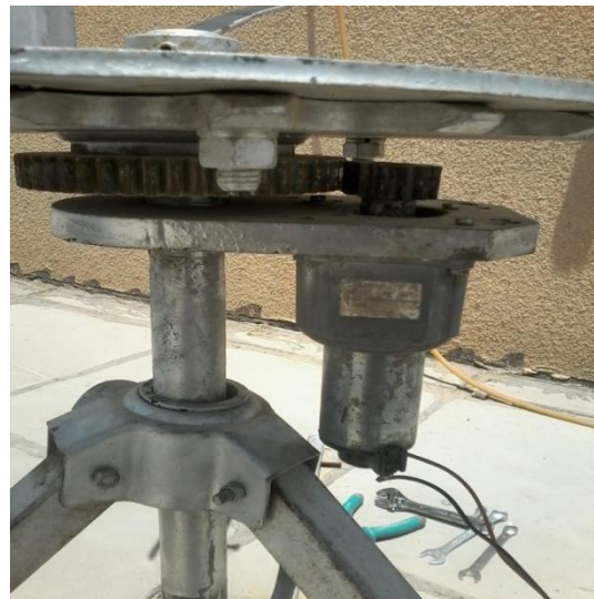
Fig. 2a. DC gear box (axial motion)
