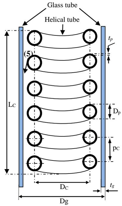
**Fig. 2.** Schematic cut-away view of a helical coil tube inserted in a glass tube.
