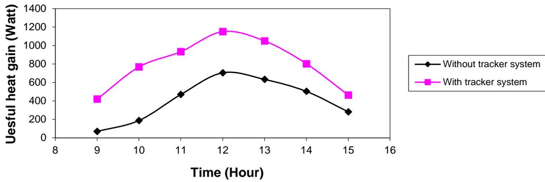
Fig. 7. Useful heat gain during daytime on (16th and 17th) April 2020
