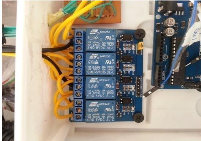
**Fig. 4.** Control circuit: connecting the relay circuit with the Arduino and motors.
